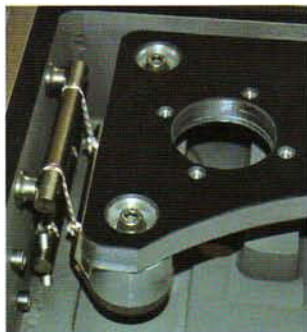
Magnetically suspended arm board, the Kevlar cords
